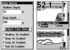
Sonar Alarms menu with Adjust Zone selected (left). Adjust Zone Alarm selection box with Upper selected (right).
